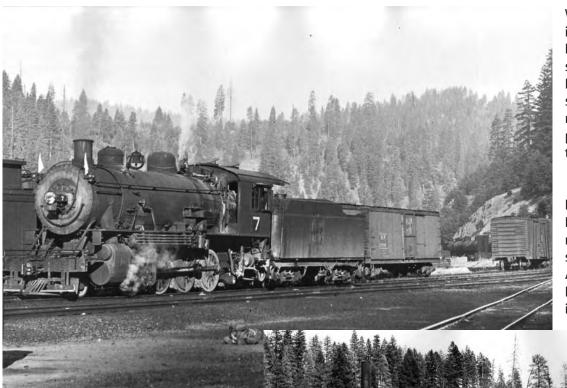
WP 7, a 2-8-0 built by Baldwin in 1906, switches a train in the Feather River Canyon, specifically at the east end of Keddie. The roundhouse, shown in the photo below, is right behind the photographer. This class of engine was the first received new by WP.
