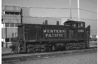
December 7, 1982 found the 1502 working the Oakland area tracks. Of interest is the mounting of the 5 chime horn on the roof in contrast to the mounting as applied to the 1503 below.
