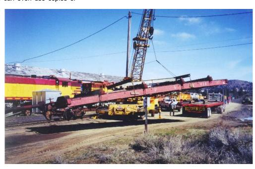
After being lifted from the truck trailer one of the flat cars is being swung around in preparation for setting it back on its arch-bar trucks.
