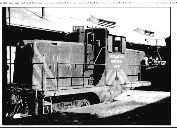
Our SN 146 shows her original paint scheme of black with orange stripes, with silver on portions of the handrails and silver foot boards, while awaiting assignment at Sacramento in the early 1950's. Note the angled number boards on the cab roof but no yellow beacon. SN Steeple Cab #653 is behind her. –Courtesy Brad Lomazzi
