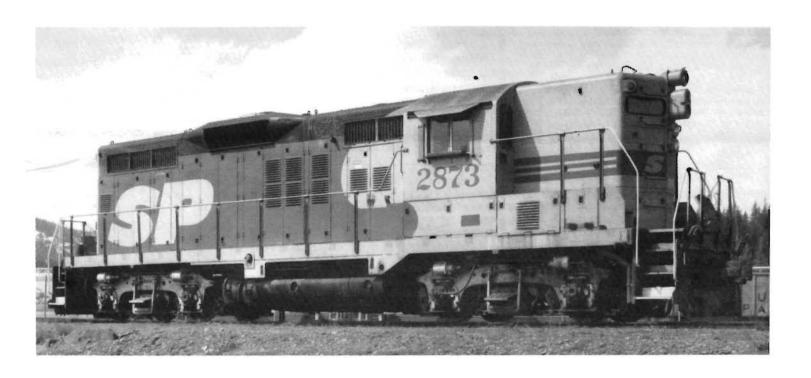
New Arrival — SP 2873 - EMD GP9E, EMD #22897, Built 12-56. Built as SP 443, upgraded and renumbered SP 3798 2-18-77, renumbered between 11-78 to 1-79 to SP 2873. It has the failed merger (SF-SP) paint scheme "Kodachrome." Photo by Ed Warren.
