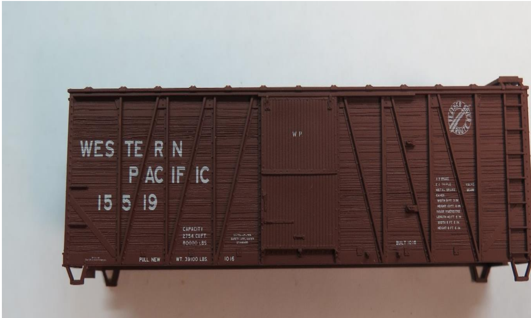
The basic body of the box car
