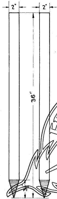
No. 5 GRADE STAKES 2"x2"x36" Rough Material: Pine To be securely tied in bundles of 25
