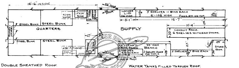
FLOOR, SIDE & END WALLS TEG LINED 8 25 X 29 CABOOSE SASH
