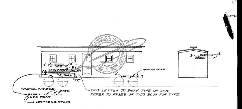
7.25.27. OFFICE CAR TYPE NEW POST NEW POST 6 ROOF JACK BUNK. BUNK LOCKER VERT. OFFICE. Z-GXG-0 TABLE. VERT.GRAD 2 DRAWERS. BUNK BUNI WATER ALL SASH 25 X 29" BOTTOM OF WINDOW FRAME OPENING WALLS& FLOOR AROUND STOVE LINED 38" ABOVE OLD FLOOR OF CAR WITH OLD CAR ROOFING APPLY 2 COATS GRAY PAINT INSIDE . TEG FLOORING LENGTHWISE , OFFICE ONLY TEG WALL LINING . BX 6-6 END DOOR SCREENS 2-0"X6-2" STEEL SIDE DOOR LADDERS CAR INSIDE 8-6 WIDE 40-0 LONG. SCALE 4=1 FT CS. 7.6.27
