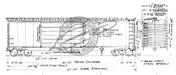
BARBER S-2-C STABILIZED TRUCKS LENGTH INSIDE \_\_ 50'-5% CAPACITY 100000 LBS WEIGHT - BODY WIDTH " 9-2/2" ..... 4840 CU. FT. RUBBER DRAFT GEARS WESTINGHOUSE TYPE ABIOIZ AIR BRAKES HEIGHT " \_\_\_\_\_ 10'-5\frac{1}{3}" TOTAL 55800 LBS
