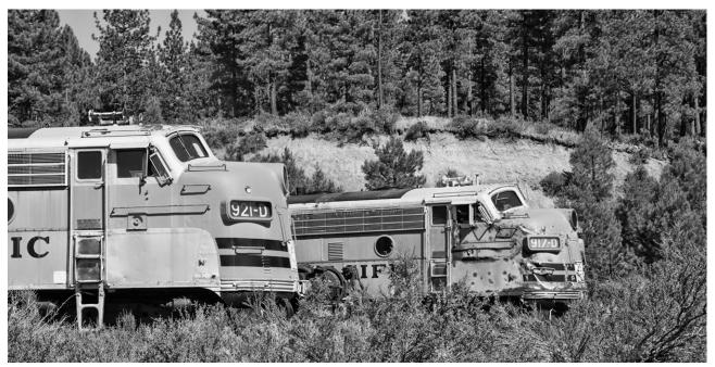
Western Pacific F7A 917-D recently returned to operation after heavy repairs. Cosmetic restoration work on the venerable covered wagon is next on the list. Here is passes sister WP 921-D near the sewer plant crossing on the day it returned to operation: June 14, 2018
