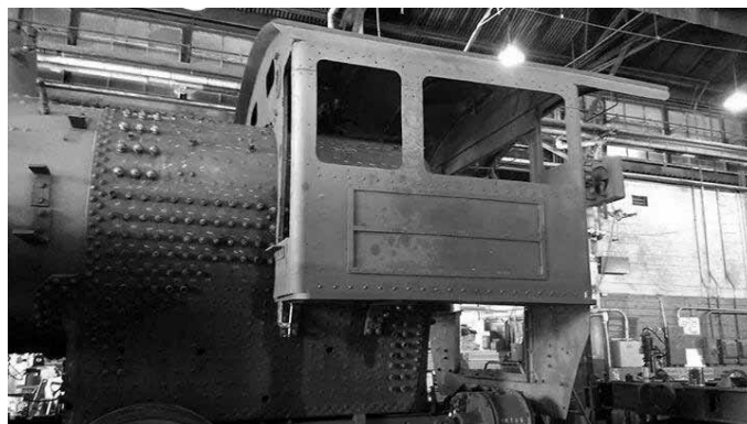
Western Pacific 0-6-0 165 has her cab back! During the work session in September, 2014, the 165 reached a major milestone with the reinstallation of the locomotive's refurbished cab.
