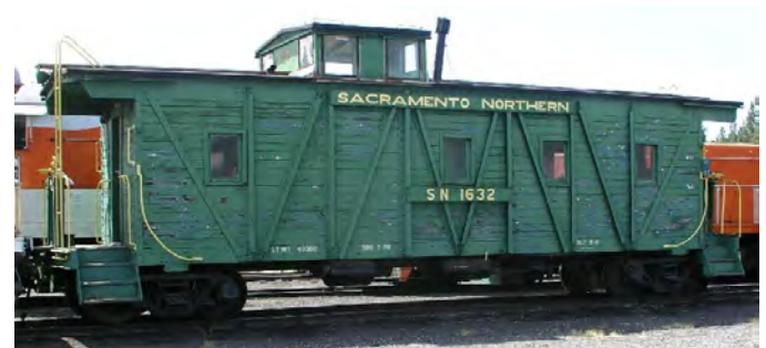
SN 1632 - a Single-sheathed cupola caboose, rebuilt from boxcar 15303 in 1938 by WP - photo by Brian McCamish
