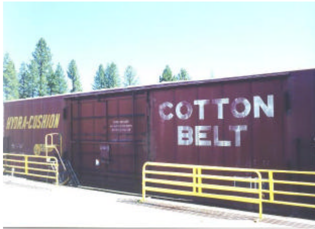
The fourteen foot plug door can be fully closed when the car is not being used. When closed the car appears normal and also adds additional protection and security for the contents. - John Walker
