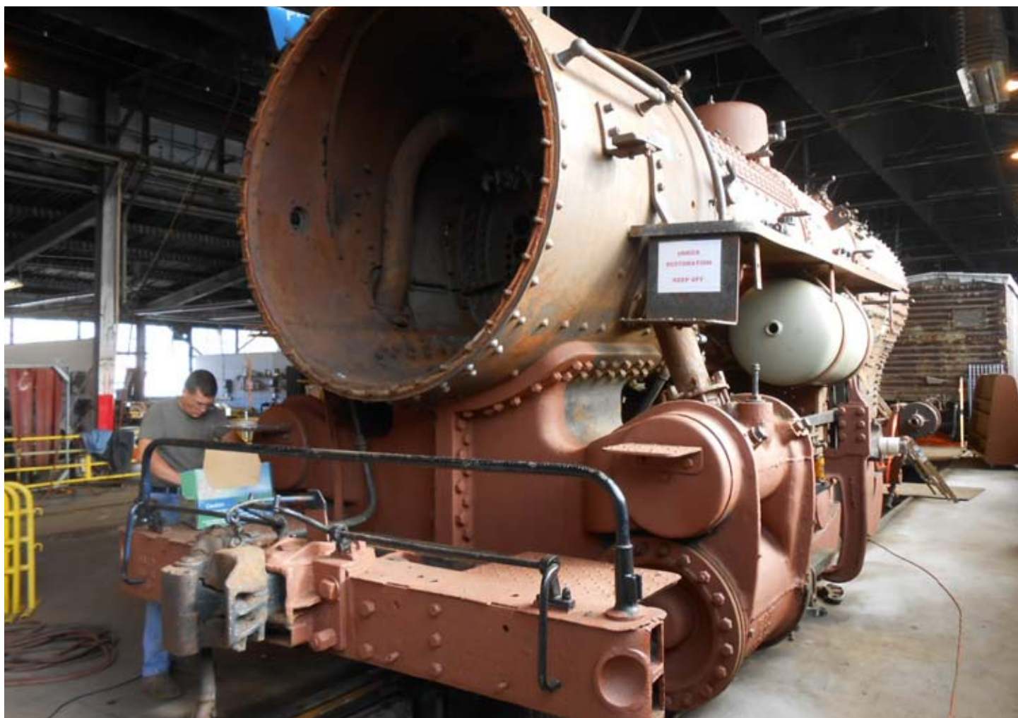
David Elems works on the front pilot of the rapidly reassembling WP 165. - Dave Roth photo
