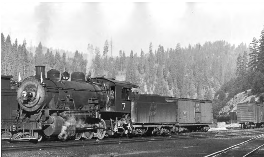
WP 7, a 2-8-0 built by Baldwin in 1906, switches a train in the Feather River Canyon, specifically at the east end of Keddie. The roundhouse, shown in the photo below, is right behind the photographer. This class of engine was the first received new by WP.
