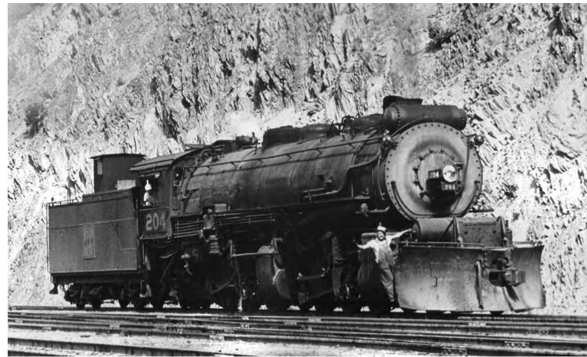
WP 204, a "Little Wamp" in WP slang, rolls through the yard at Keddie. These 2-6-6-2 Mallets were fixtures in the Canyon until they were displaced to the NCE by the arrival of the 2-8-8-2 simple articulated locomotives, "Big Wamps".
