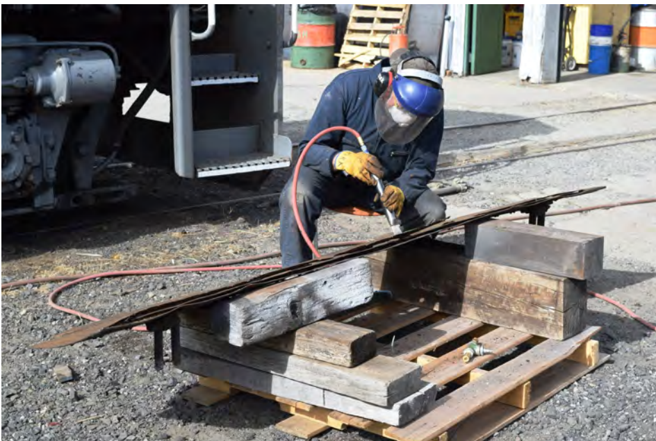
Kirk Baer seen here scaling the deck plate for the 165 next to the WP 1503. - photo by Greg Elems
